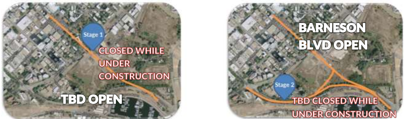
Graphic 1. Construction staging and road closures
